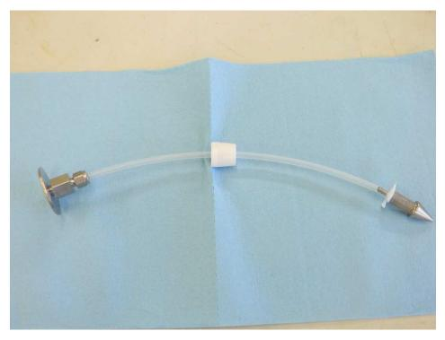
Picture #3 – Soil vapour insert with attached PTFE sampling tubing
