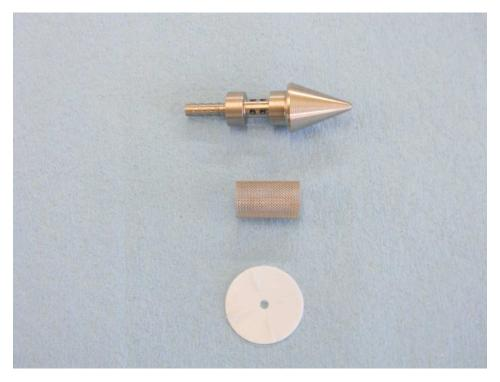
Picture #1 – An example of the stainless-steel soil vapour insert, PTFE umbrella, and stainless-steel mesh to be used for an installation of the soil vapour monitoring points
