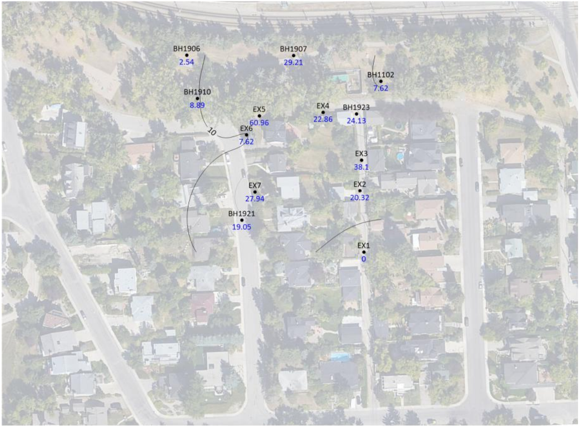
Header 1305 (EX2, EX3) On, 12 Hours, Units of Vacuum in mm of Water
