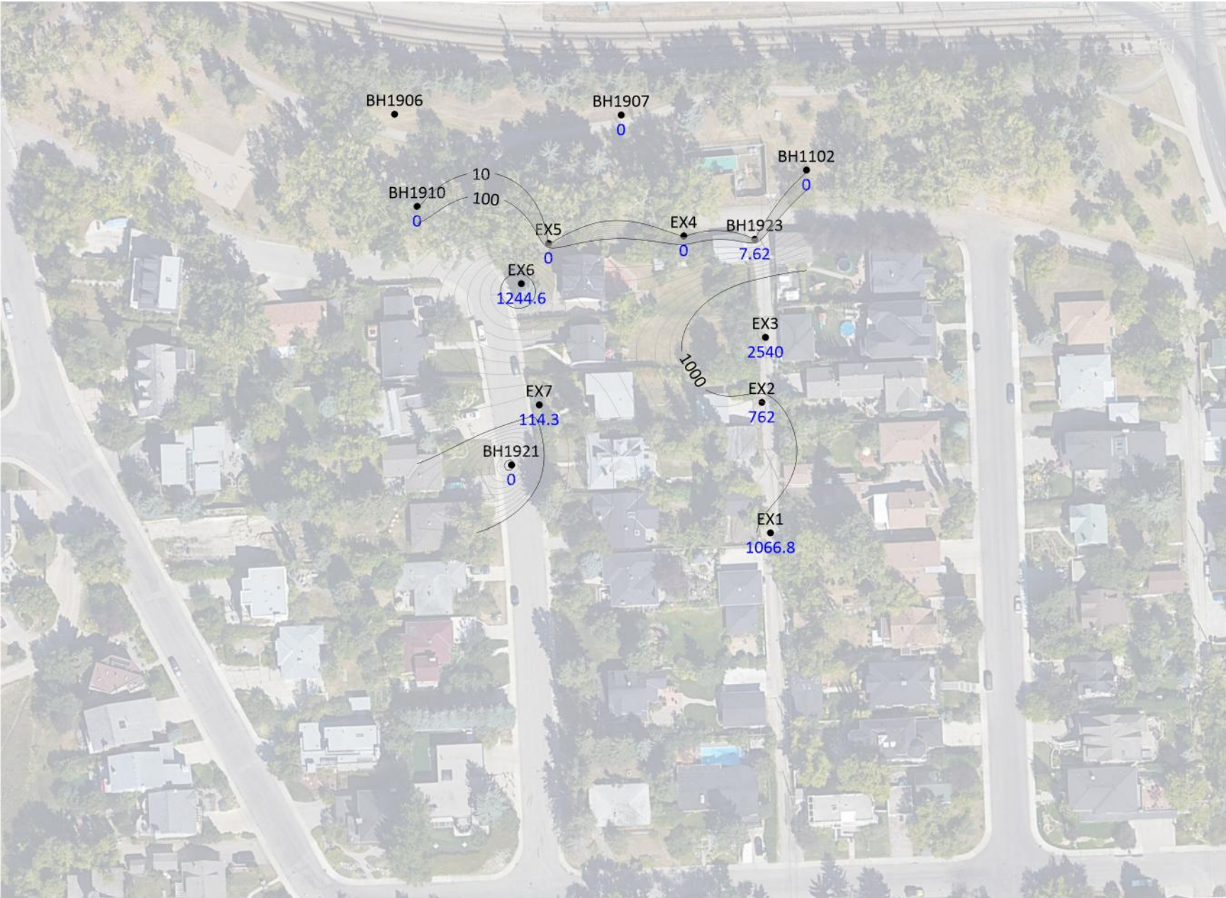
Headers 1305 (EX2, EX3) and 1307 (EX1) On, 30 Minutes, Units of Vacuum in mm of Water
