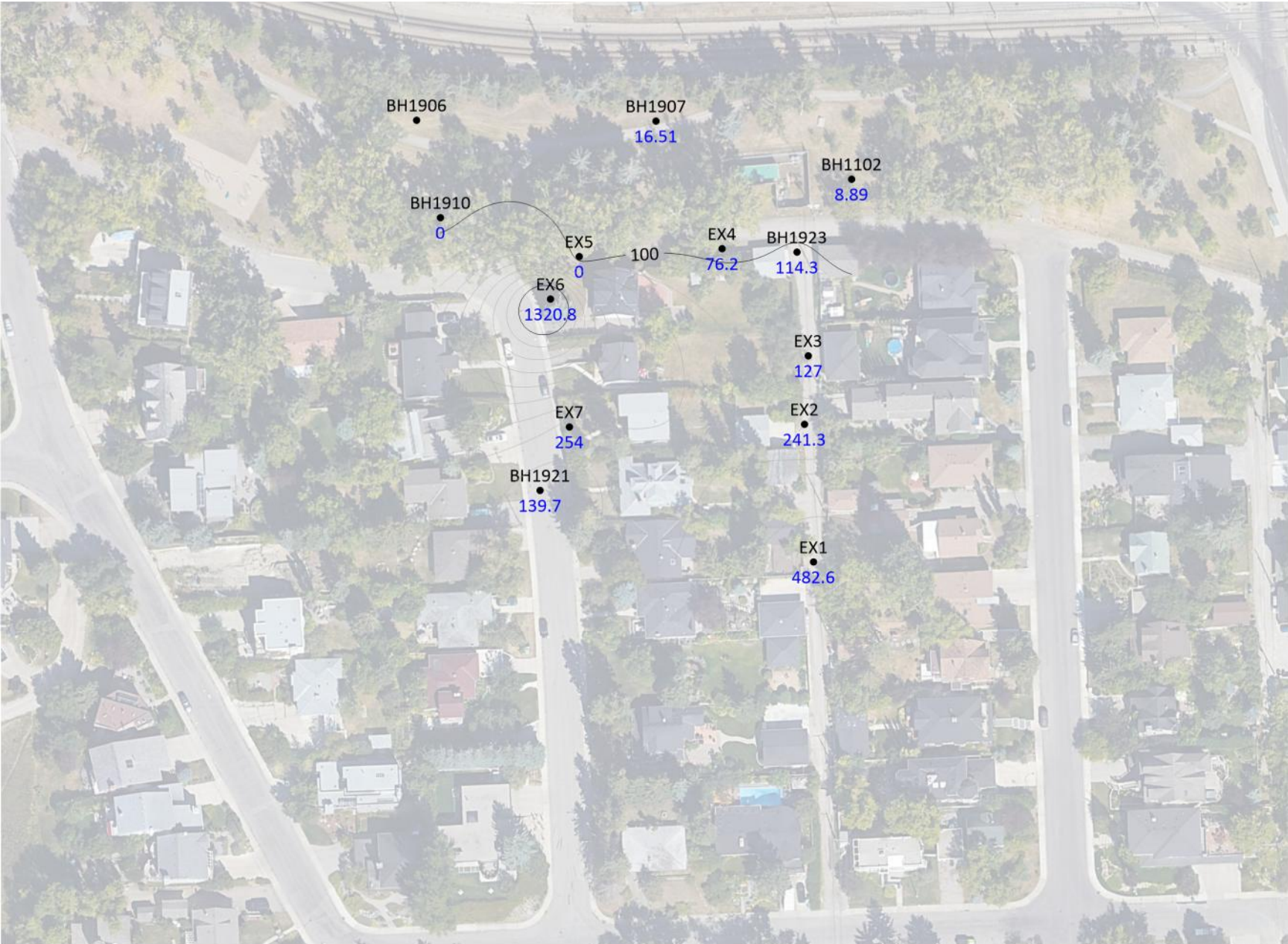
Headers 1305 (EX2, EX3) and 1307 (EX1) On, 24 Hours, Units of Vacuum in mm of Water
