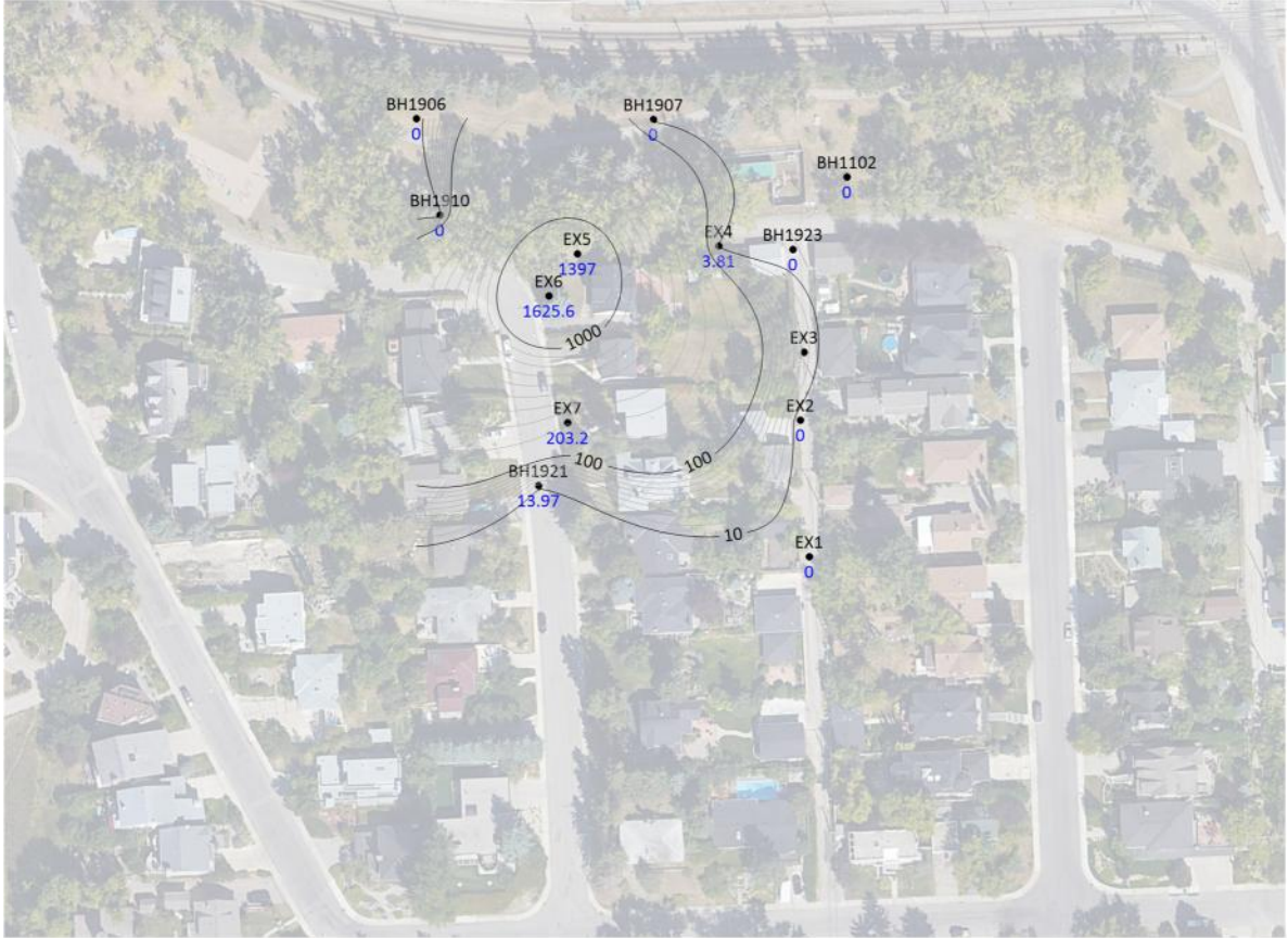
Headers 1301 (EX6, EX7) and 1303 (EX4, EX5) On, 24 Hours, Units of Vacuum in mm of Water
