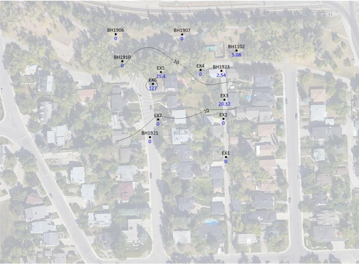
Header 1305 (EX2, EX3) On, 30 Minutes, Units of Vacuum in mm of Water
