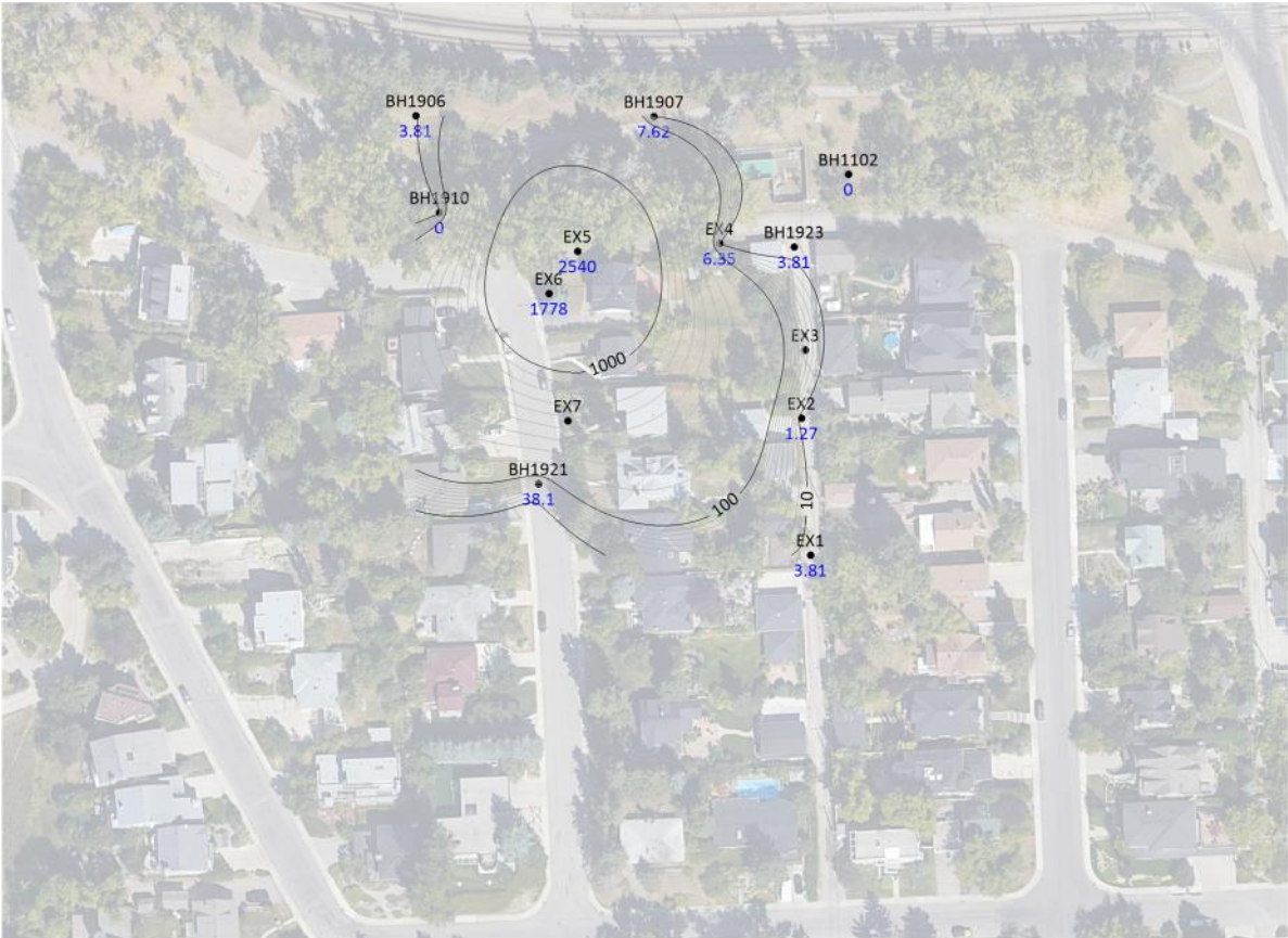
Headers 1301 (EX6, EX7) and 1303 (EX4, EX5) On, 30 Minutes Units of Vacuum in mm of Water
