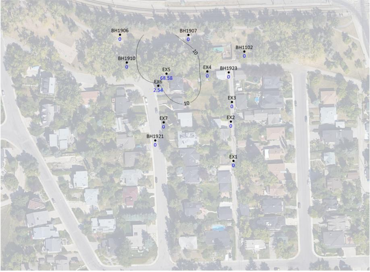
Header 1305 (EX2, EX3) On, 24 Hours, Units of Vacuum in mm of Water
