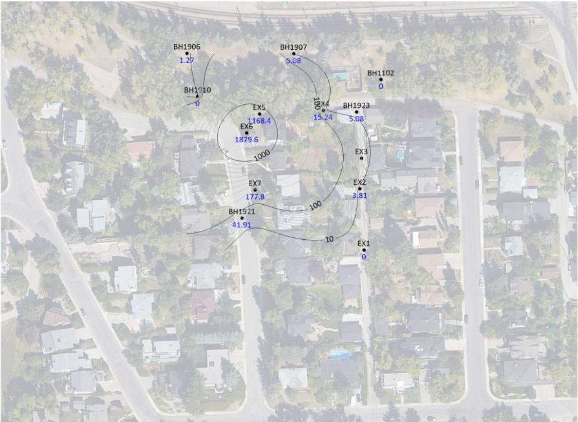
Headers 1301 (EX6, EX7) and 1303 (EX4, EX5) On, 12 Hours, Units of Vacuum in mm of Water
